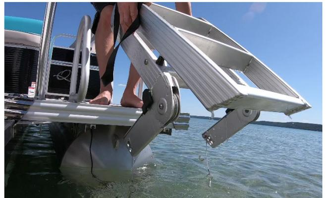
REVO Ladders are designed to exceed industry standards. Each ladder is built with heavy wall aluminum extrusions, robust (internal) stainless-steel cables, and stainless hardware. In addition, the ladder is self-draining, eliminating the ability to freeze and crack.
