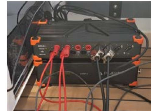
Figure 2. SIRIUSi HS 4x HV, 4x LV with DS-BP2i. Measurement Setup
